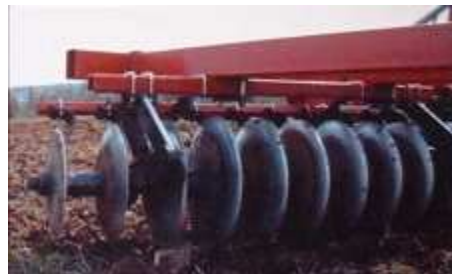
Coil flex gang system for superior protection
